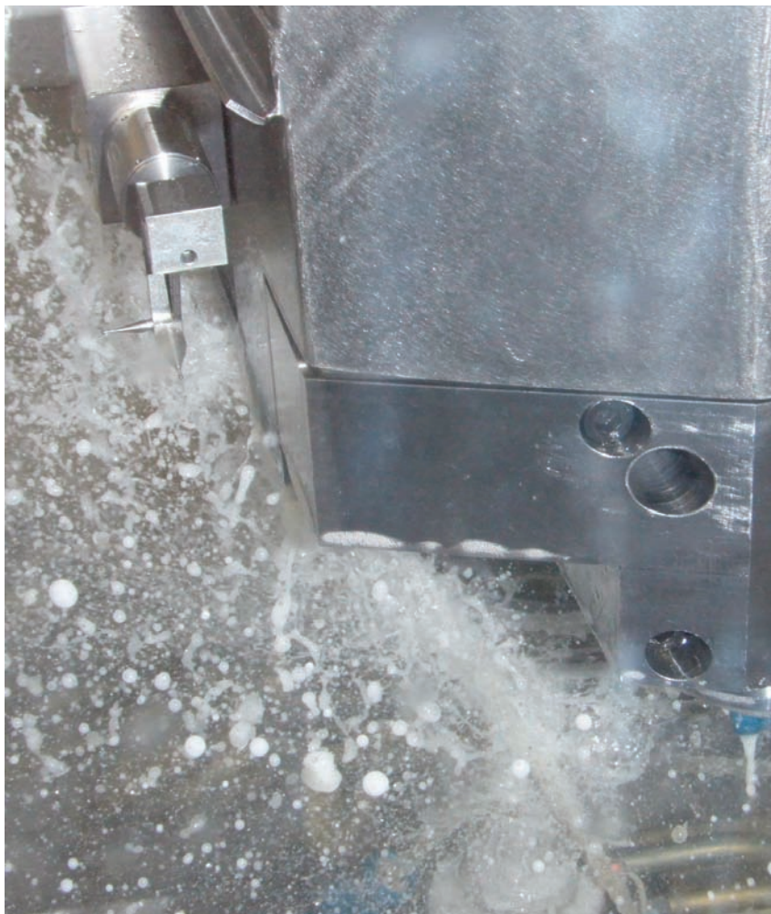
m&h touch probes are continuously covered in coolant and abrasive particles.
