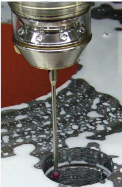
Determining position and fit size with 3D Form Inspect
