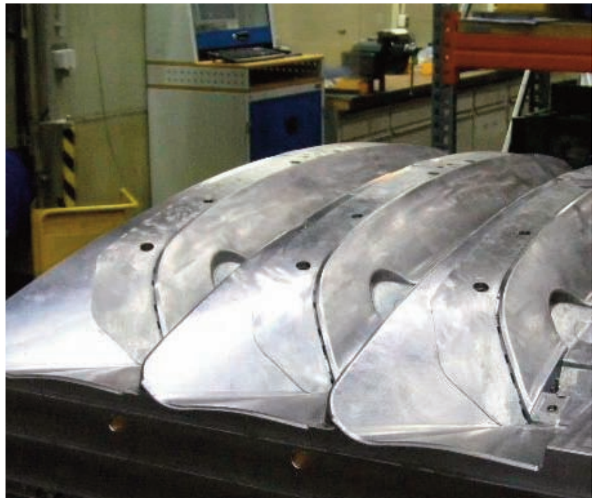
Free-form surfaces on mould cores for VW vehicle parts are measured using 3D Form Inspect.
